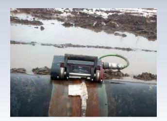
The GW-4 works with an internal panoramic CP X-ray source and can complete a 3-inch wide, high-resolution scan of a 24-inch pipeline in 2-3 minutes depending on pipe wall thickness and source power.
