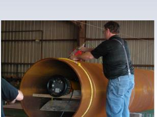
The GW-4<sup>™</sup> is an automated digital X-ray scanner for inspecting circumferential pipeline and vessel welds. The magnetic scanner travels directly on 12" dia. and larger pipe.
