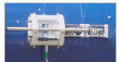
MagScan Scanning on painted pipe using 2 off PA probes
