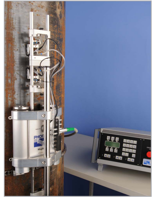
MagScan configured for ToFD inspection
