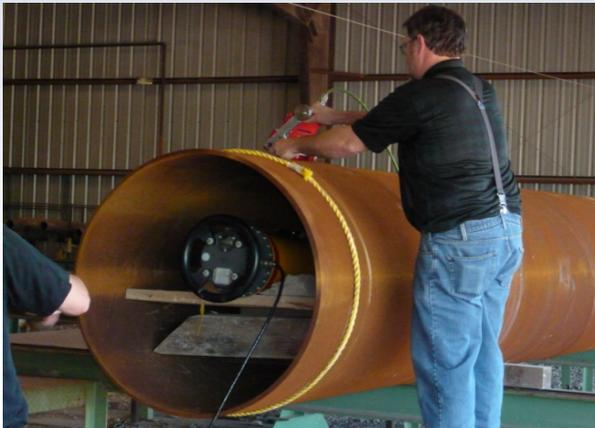
The GW-4 works with an internal panoramic CP X-ray source and can complete a 3-inch wide, high-resolution scan of a 24-inch pipeline in 2-3 minutes depending on pipe wall thickness and source power.
