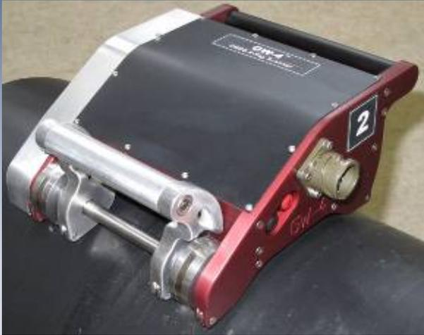
The GW-4™ is an automated digital X-ray scanner for inspecting circumferential pipeline and vessel welds. The magnetic scanner travels directly on 12" dia. and larger pipe.
