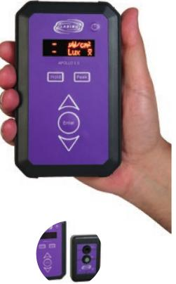
✓ Wireless Sensor measures up to a distance of 16 feet (5 meters) from the Reader unit
