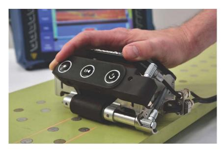
R-Evolution is an ultrasonic array probe housed in a lightweight water-filled roller, delivering fast immersion quality C-scan inspections in the palm of your hand.
