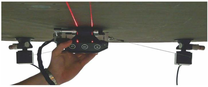
R-Evolution has a single axis encoder for inspecting C-scan strips or can be attached to the Phoenix Tracer for a versatile and portable large area C-scan inspection system.
